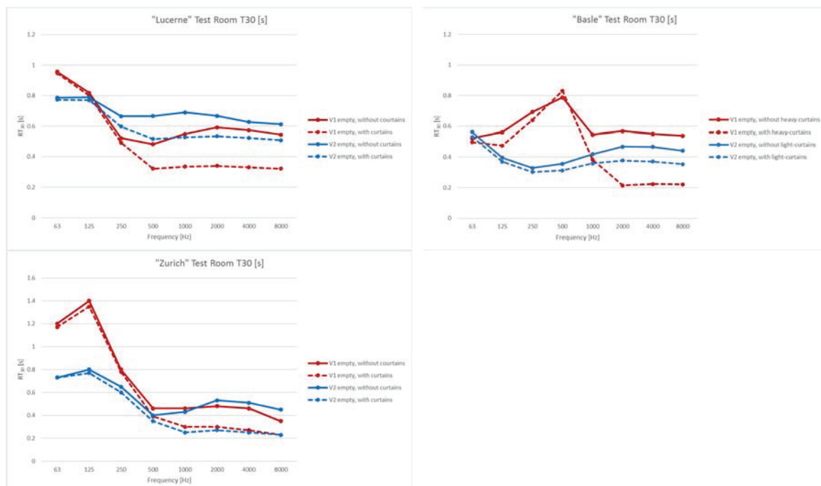
Figure 4 – Reverb Times of the three test-rooms (blue curves show Version 1, red curved show Version 2, dotted lines show respective reverb times with acoustic curtains in full use)
