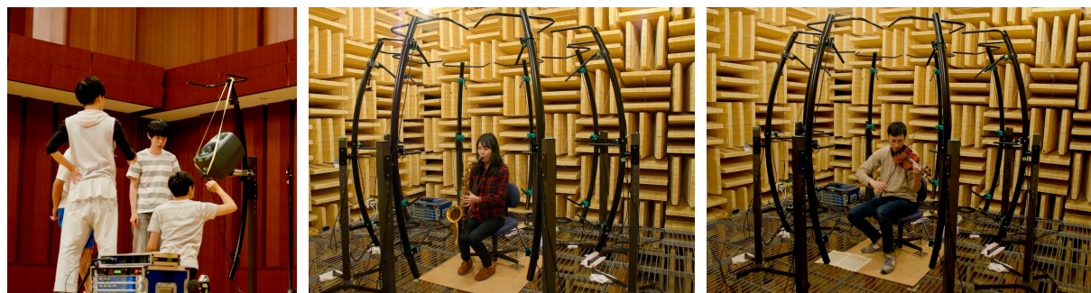
Figure 6: Measurement of impulse responses with a slanted loudspeaker (left) and recordings with 24-channel narrow-directional microphones for the saxophone (center) and violin (right).
