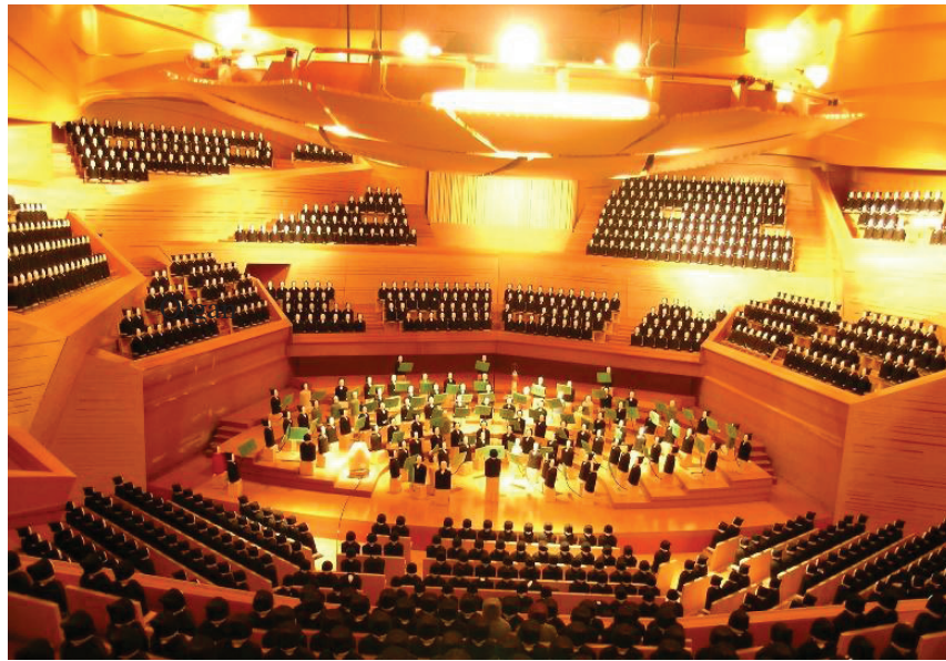
Figure 6 - DR concert hall 1:10 scale model with “orchestra” for stage acoustic measurements
