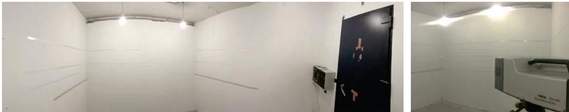
Figure 2 – Experimental setup. Left: 360-degree view of the room in which the measurements were performed. Right: Scanning laser vibrometer used to perform the measurements.
